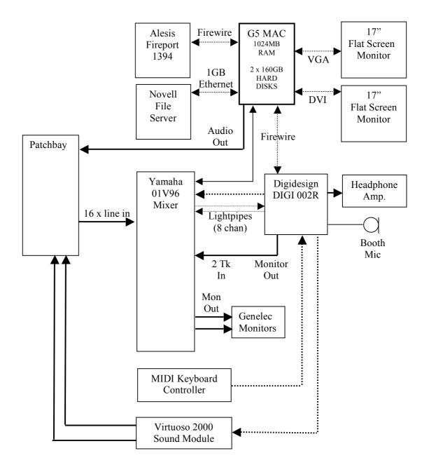
Note 1: Audio is routed from the 01V96 to the DIGI002R via the Lightpipe optical interface.
